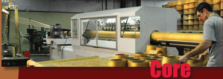
Western Container has upgraded their offerings to include precise strapping cores cut in-line with their new Multi-knife Winder/Cutter. Precise lengths are controlled by having multiple knife holders where material is cut in-line between these servo driven knife holders. Accuracy is paramount on this new machine with in-line cutting tolerances of .020, for the most stringent of applications.
